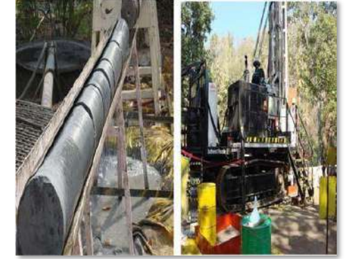
Large Diameter Kimberlite core (8”) for Rio Tinto at Bunder, MP – Drilled by BLY LF230 upto a depth of 352 Meters. Largest coring done in India till date
